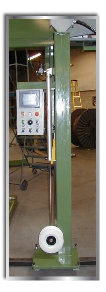
Dancers are primarily used for speed regulation of winding or unwinding equipment. They can act as the primary mode of regulation, or as a trim to another speed reference. They can be linear or pivoting for inline applications, or articulating for applications whereby the product fleets offline. They are usually used in slower line speed applications.
